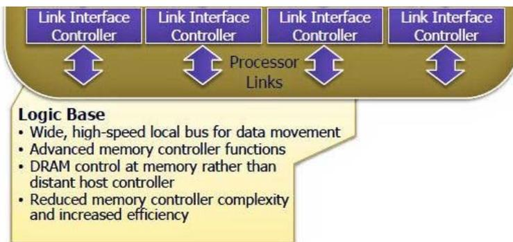
The reason Micron felt the need to take this design approach is because large DRAMs (and other semiconductor memories) are bandwidth-constrained by the limited number of interface pins. The consequence of pin limitations in memory design is the need to perennially push transfer rates into the GHz range. One way to solve this problem, taken by the JEDEC Wide I/O committee, is to adopt a very wide interface—512 data bits in the case of Wide I/O.
