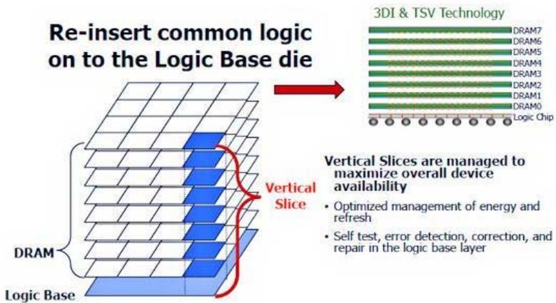
This stack then sits atop a "logic chip" that contains memory controllers for each DRAM array stack plus SERDES interfaces to connect the HMC to a host processing complex. Here's a block diagram of logical design of the HMC:
