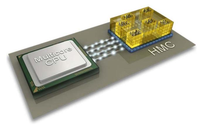
The current prototypes either have 128 or 256 memory banks available to the host system and the first HMC spec will reportedly offer 2GB and 4GB packages that provide bi-directional bandwidth of up to 160GB/s, according to a Micron exec.
